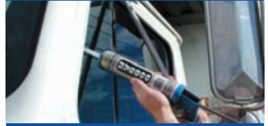
Adhere weatherstripping to windows.
